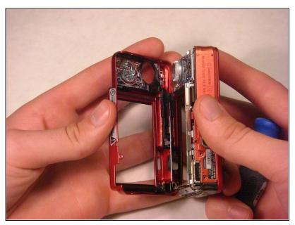
• After detaching the back cover, carefully pull it off.
