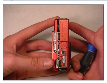
Gently detach the back cover by holding onto both sides of the camera and pulling them apart.
