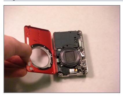
Fully remove the front casing from the camera and set it aside.
