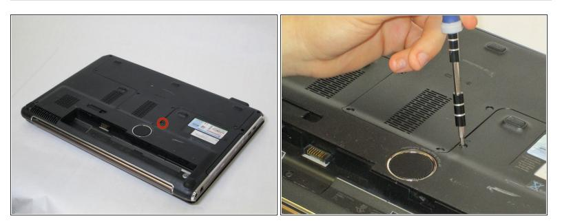
Remove the single PM2.5x7.0 screw from the bottom panel.
