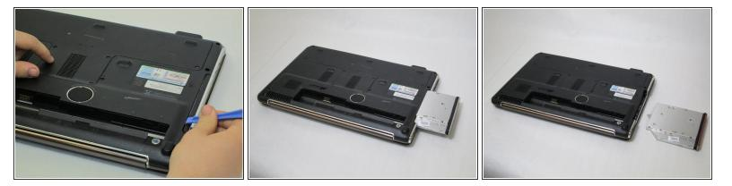
Pull the drive out of the right side of the device using the plastic opening tool.
