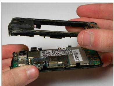
Using the spudger, pry off the back body panel by wedging the spudger in between the front and back panels on the side face. Remove the back body panel.
