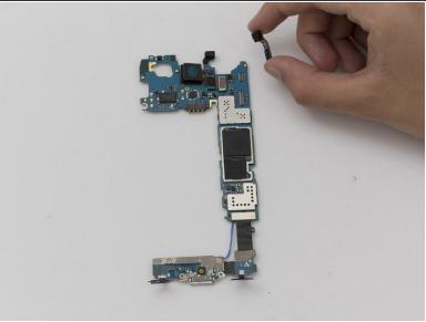
Use the plastic opening tool to gently remove the ribbon cable connecting the front camera to the motherboard. To reassemble your device, follow these instructions in reverse order.
