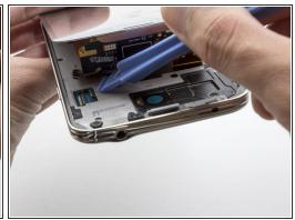
Start lifting the screen from the top. You will see a black ribbon cable attaching the display to the motherboard. Use the plastic opening tool to lightly detach the connector.
