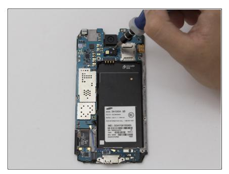
Remove the single silver 4 mm screw from below the rear camera with a Phillips#00 screw driver.
