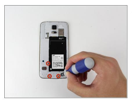
Flip the device over and remove the three 5mm screws with a Phillips#00 head screw driver.
