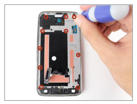
Unscrew the ten 4 mm screws from the midframe with a Phillips#00 head screw driver. You may want to use tweezers or a magnetic screwdriver to remove them.
