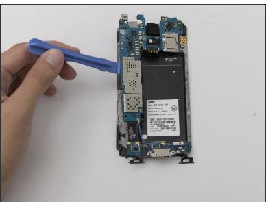
Gently lift the motherboard off of the second midframe with the plastic opening tool.
