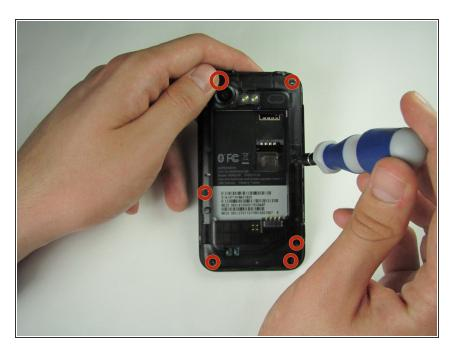
Remove the seven 1.42 mm Torx T5 screws
