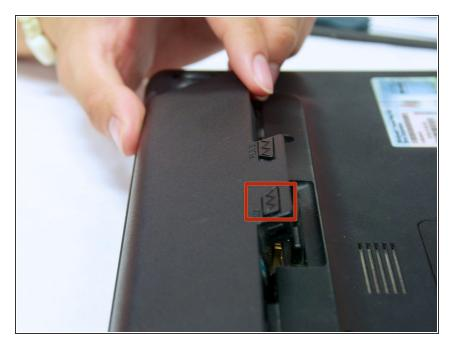
Push and hold the right-hand switch, which says "release" above it, and lift the battery up out of its place.
