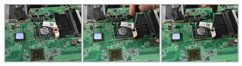
Remove the the black screw above the processor with a flathead screwdriver.
