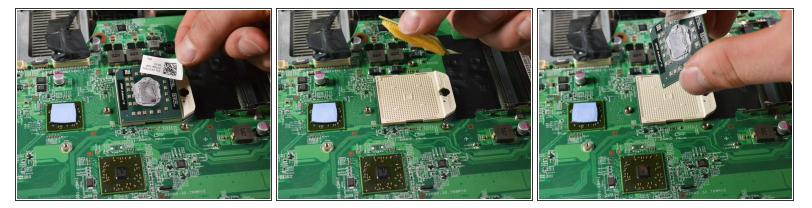
• Grab the sides of the processor with your thumb and forefinger to remove the processor.
