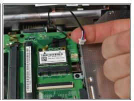
Disconnect the white block of wires which is the right-most wire connecting the covering to the laptop.
