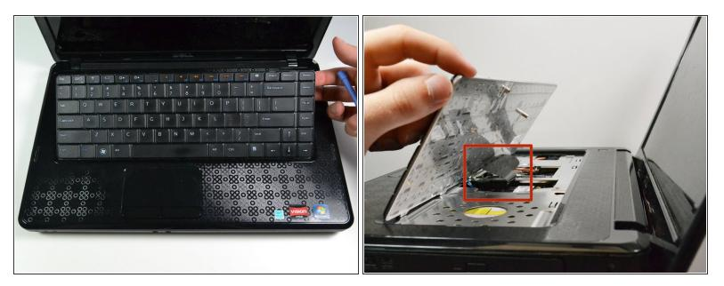
• After the top edge of the keyboard is loose, pull up on the keyboard gently.
