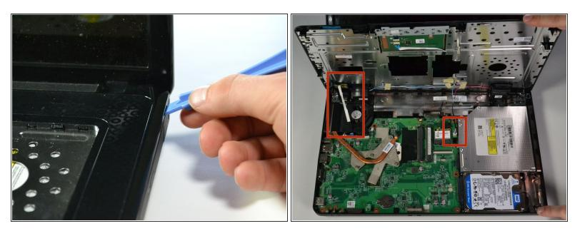
Use a plastic opening tool to pry up the plastic covering of the laptop by wedging it underneath one side of the covering and lift up.
