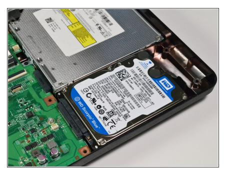
• Locate the hard drive in the bottom right-hand corner of the laptop.
