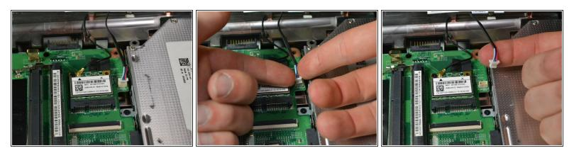
Disconnect the white block of wires which is the right-most wire connecting the covering to the laptop.
