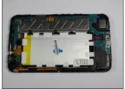
Working slowly and carefully, move around the entirety of the face of the device. Small plastic clips should release, if not, apply gentle outwards pressure until you hear the clips popping off.
