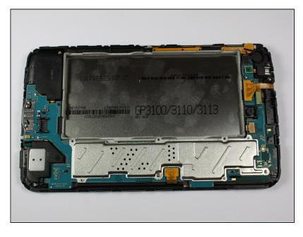
To finish battery replacement, place your new battery where the old battery was in your device, as shown in the picture.
