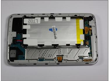
• With a plastic opening tool, gently insert the prying end in between the glass digitizer and the silver frame from the front of the device.
