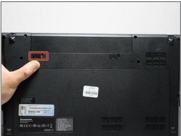
• To unlock the battery, flip the laptop over so that the bottom is facing upward. Then unlock the left clip by pushing the clip to the left.
