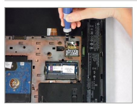
Use a Phillips #1 screw driver to unscrew the black 4 mm Phillips #1 screw on the wireless card.
