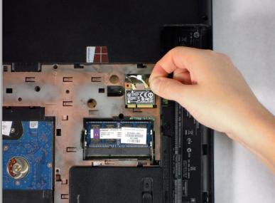
Use a plastic opening tool to lift the wireless card out of its slot.
