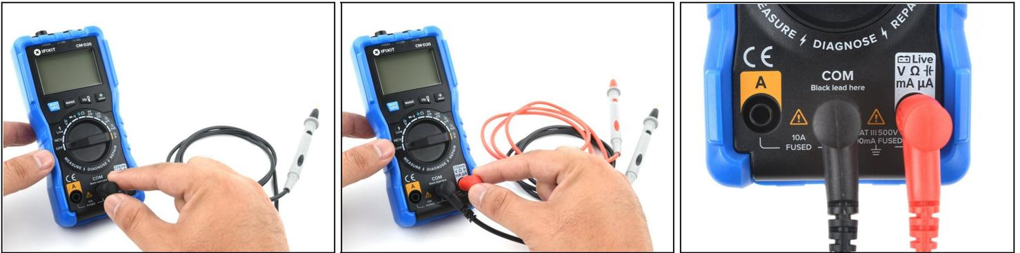
⚠ To begin, make sure no current is running through the circuit or component you want to test. Switch it off, unplug it from the wall, and remove any batteries.
