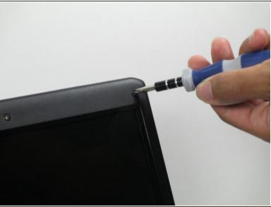
Remove the six 2.0 mm Phillips #1 screws from the perimeter of the bezel.
