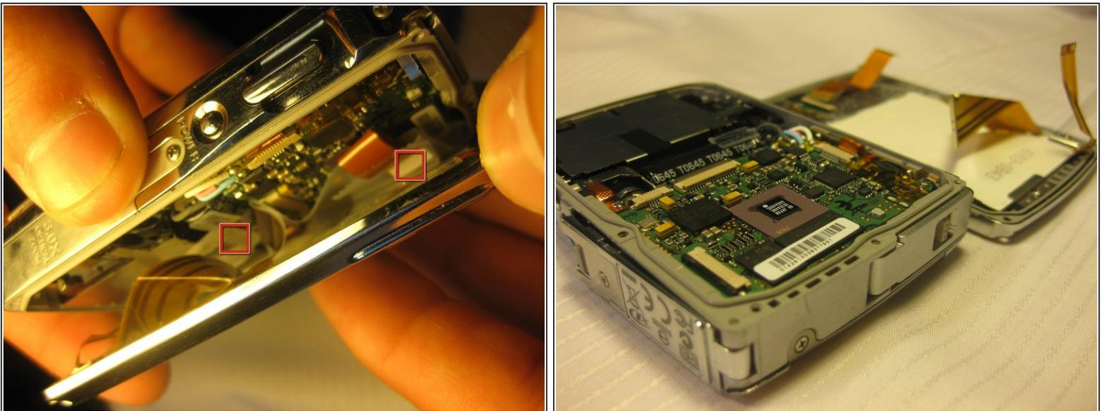
**⚠ Be careful when removing the back cover; you will need to detach the connecting ribbons. Use tweezers if necessary.**
