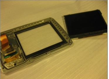
• Use <u>tweezers</u> to remove the loosened LCD screen.
