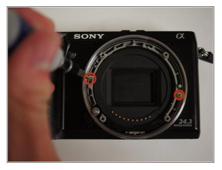
Remove the two newly visible #00 screws within the metal ring.
