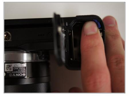
• With the battery door open, push the blue lever in the battery compartment to release the battery.
