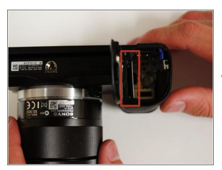
To the left of the battery compartment, the SD card needs to be pushed down slightly with your
