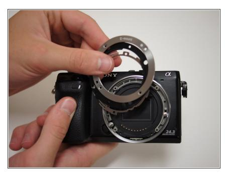
• Remove these three layers from the lens mount with your finger or by turning the camera face down.
