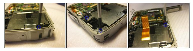
Unscrew four 2mm long screws using the #00 Phillips screwdriver.
