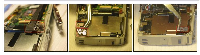
Remove four metal tabs from corners where the 2mm long screws were attached using tweezers.
