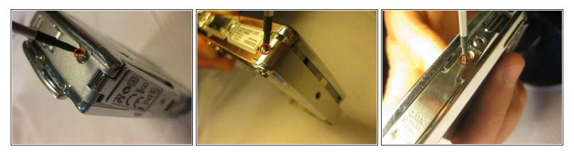
• Using a #00 Philips Head Screwdriver, remove the screws located on all four sides of the camera.
