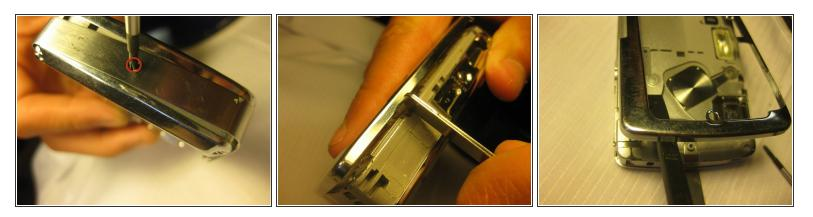
• After removing all four of the screws, pry the side covers off of the camera.
