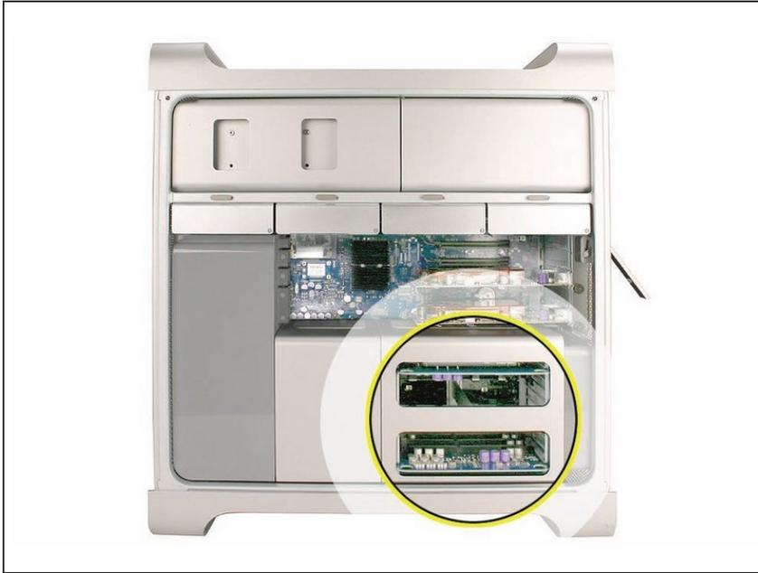
**Warning:** Always wait 5–10 minutes for the computer to cool down before you remove or install memory. The DIMMs may be very hot.
