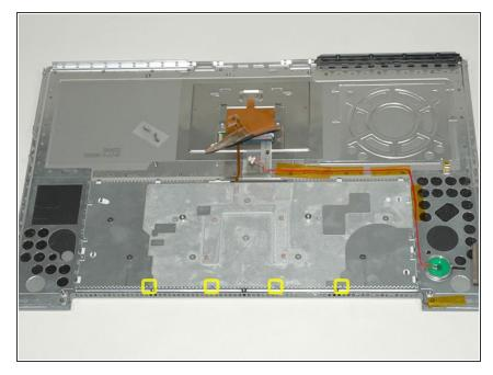
There are four locking tabs along the back edge of the keyboard holding it in place. These tabs must be straightened before you can remove the keyboard.
