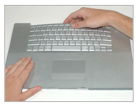
Maintaining your hold on the keyboard, lay the casing flat and gently bow the keyboard until the two tabs on either side of the keyboard come free.
