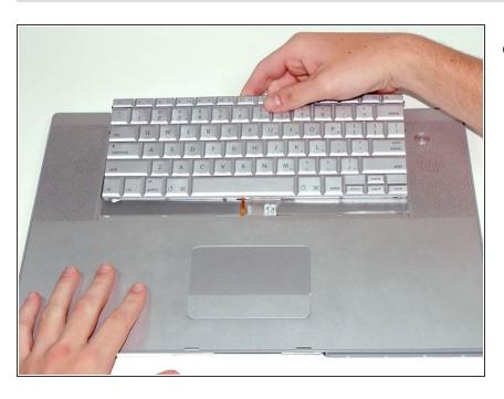
Slide the keyboard away from the trackpad and out of the upper case.
