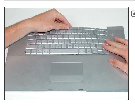
To replace the keyboard, first slide the bottom tabs in, then bow the keyboard out and slide in first the tabs on the right side of the keyboard and then the tabs on the left side.
