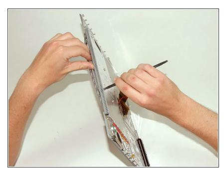
Place the upper casing on edge and use a spudger to push the keyboard away from the casing, poking the spudger through the central keyboard screw hole. Grasp the keyboard as it separates from the casing.
