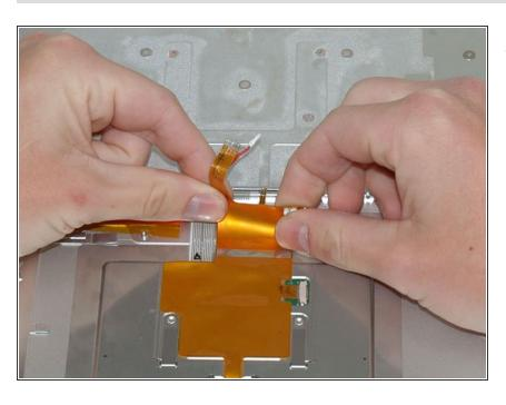
Carefully grasp both sides of the large orange ribbon cable and gently peel the ribbon up from the upper case.
