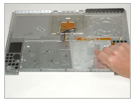
Peel back the clear plastic shielding covering the keyboard screws.
