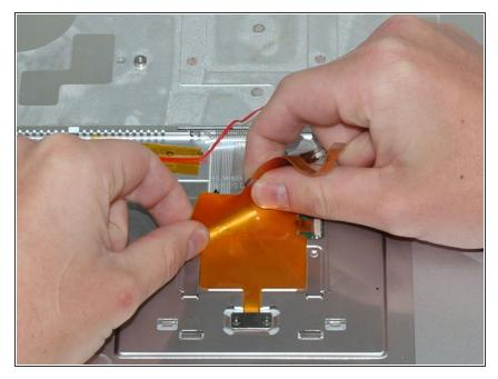
Continue to peel up the orange ribbon cable, being especially careful at the corner where the cable widens.
