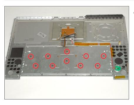
Remove the 10 identical Phillips screws attaching the keyboard to the casing.
