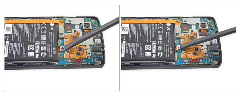
• Use the flat end of a <u>nylon spudger</u> to disconnect the battery connector.
