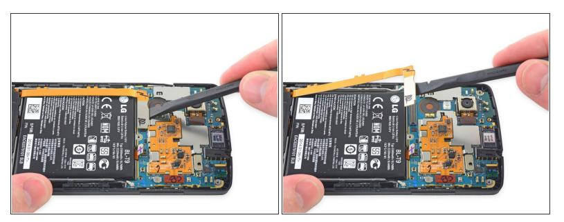
Use the flat end of a spudger to disconnect the daughterboard ribbon cable and pull it away from the battery.
