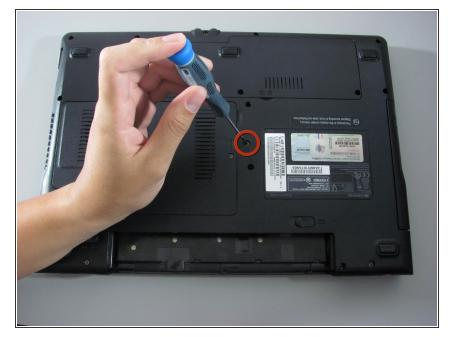
Unscrew the marked 5.9 mm Philips screw.
