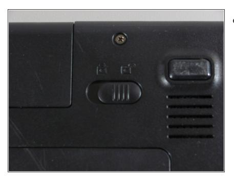
Move the latch to the right of the battery to unlock.
