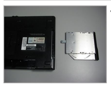
The disk drive should easily detach and can now be replaced.
