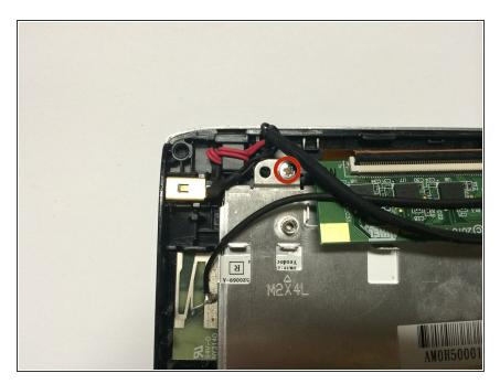
Find and remove the silver 5mm screw holding down the metal cover opposite the USB port.
