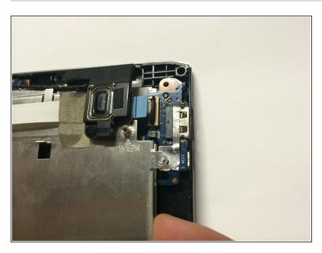
Pull up the metal panel just enough to allow access, then remove the USB port.
