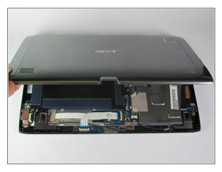
Once you have successfully pried the spudger in between the front case and back case, continue do so around the entire tablet until the back case is completely disconnected.
