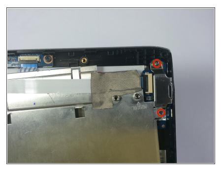
After setting aside the battery, remove the two 5mm screws holding the metal plate over the USB port.
