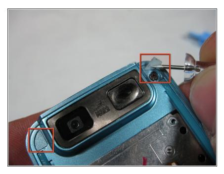
Remove the 2 screw covers next to the speaker with a push pin next to the camera.
