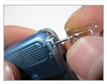
Remove the 2 screw covers next to the rear speaker with a Push Pin.
