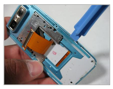
Use the ipod opening tool to pry the screen casing and the slider mechanism apart from each other.
