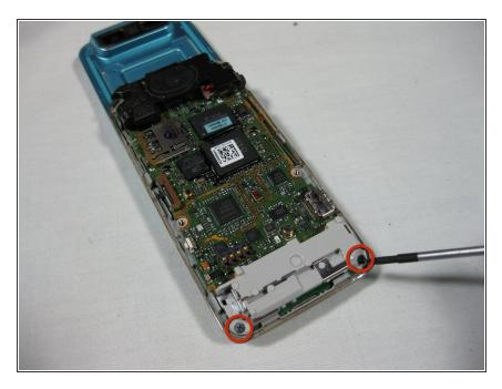
Remove the 2 screws from the back of the phone with a Phillips #00 Screwdriver.
