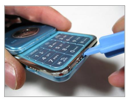
Continue sliding the iPod opening tool around the seam of the casing to separate the front and back casings.
