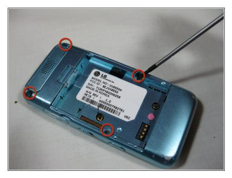
Remove the 4 cover screws with a Philips #00 screwdriver.
