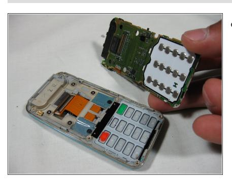
Remove the motherboard from the front casing by lifting straight up.
