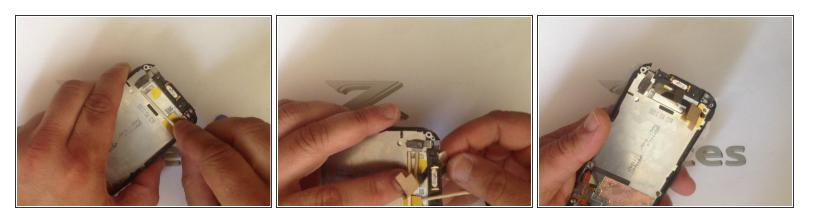
• I use toothpicks and hot air to make place for the cable of the new spare part.
