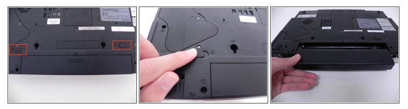
Make sure device is off and power supply is disconnected.
