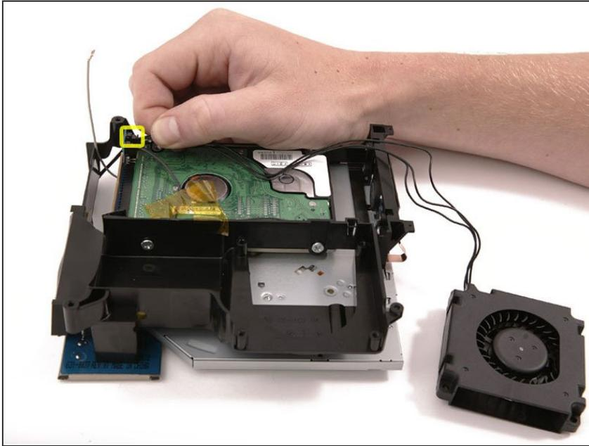
**⚠** The cable you're about to remove is very fragile - do not pull directly on the wires. Instead, try to pry up the connector directly, using your fingernails or a small flathead screwdriver if necessary.
