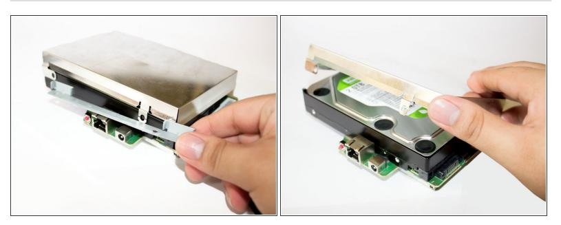
• After removing the metal clips and bars, we can now remove the shield covering the Hard Disk.
