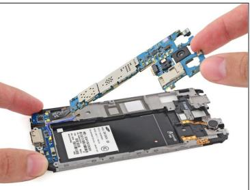
• Pull, but do **not** remove, the camera end of the motherboard up from the midframe to allow access to the connectors on the rear.
