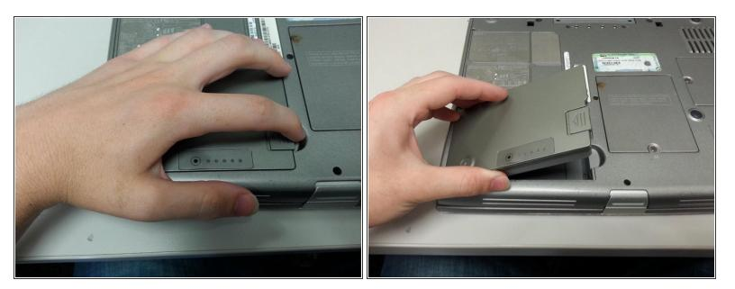
• Pull the tab to release the battery
