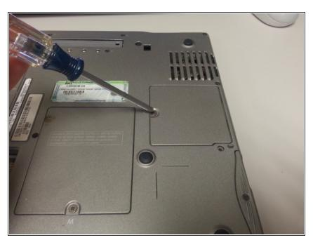
• Use your screwdriver to unscrew and lift up the panel on the right labeled with a C
