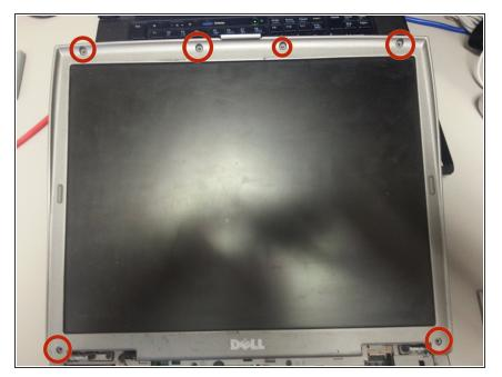
Remove the 6 screws underneath the rubber things - located in red
