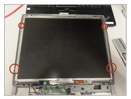
Remove the 6 screws holding in the display screen
