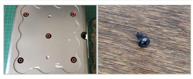
Now remove the 5 Philips screws on top
