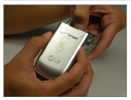
With the button unlocked, grab the battery on the sides and pull up, then slide the battery up to completely remove it from the phone.
