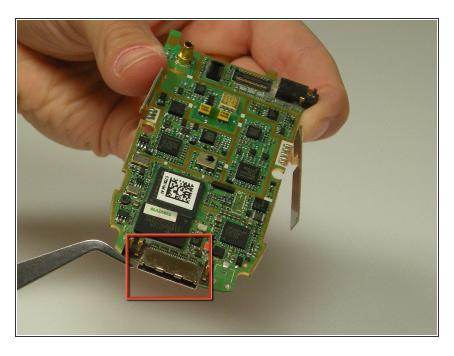
• Replace logic board to replace charging adapter.
