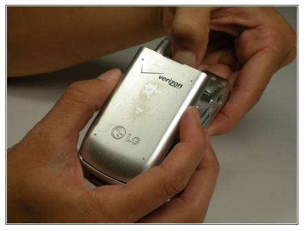
With the button unlocked, grab the battery on the sides and pull up, then slide the battery up to completely remove it from the phone.
