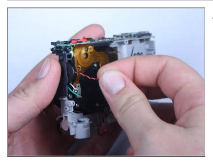
• Carefully pull the red and black wires located on the side of the camera connected to the speaker.
