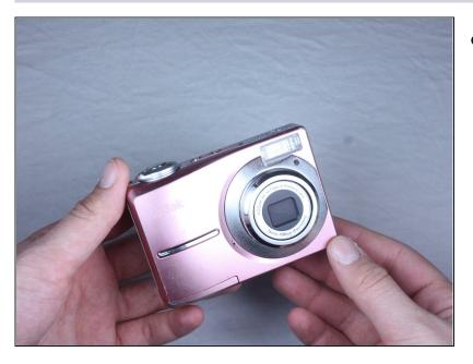
Before removing back cover, it is advisable to use an <u>anti-</u> <u>static wrist strap</u> to prevent damage to electronics.
