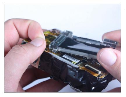
Remove the medal housing from the logic board by carefully peeling the yellow tape off of the metal housing.
