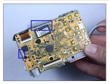
• Desolder the remaining 20 solder joints connecting the logic board to the camera.
