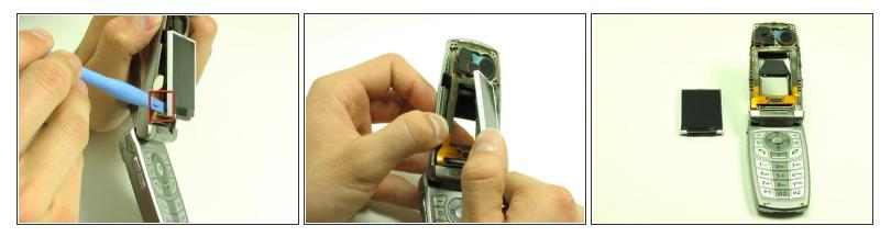
Carefully lift the LCD screen and peel it from the gold ribbon. The sticky connection runs all the way around the LCD screen.
