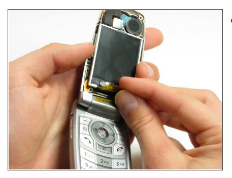
• Remove the tape from the bottom of the LCD screen.
