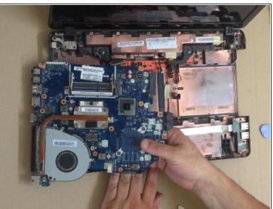
Disconnect the Power /Charging cable connector from the back side of the Motherboard.
