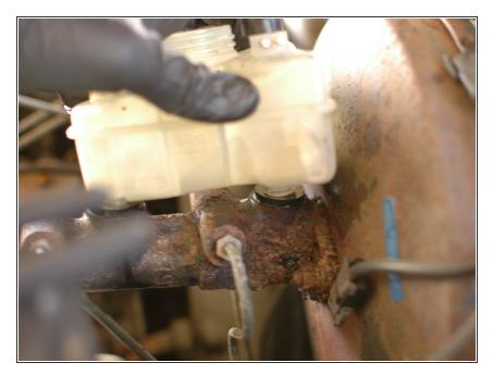
Once the front of the reservoir is inserted you can rotate the rear end in to place and push it in to the plug.
