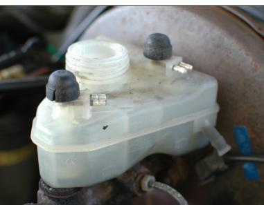
Now you can proceed to remove the reservoir. Start by unplugging the two sensor wires from each
