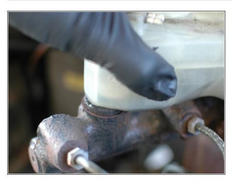
With the sensor plugs disconnected you can simply pull the reservoir out of the master cylinder. Pull straight up. It may take some force. You will have a bit of brake fluid drip and splash at this point - have a bit of water ready to rinse it off the painted surfaces underneath.
