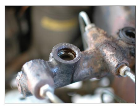
• In this picture the front plug has been removed. Proceed to carefully clean around this area with a shop towel. Do not allow dirt to enter the master cylinder - clean so that the dirt goes out, not in.
