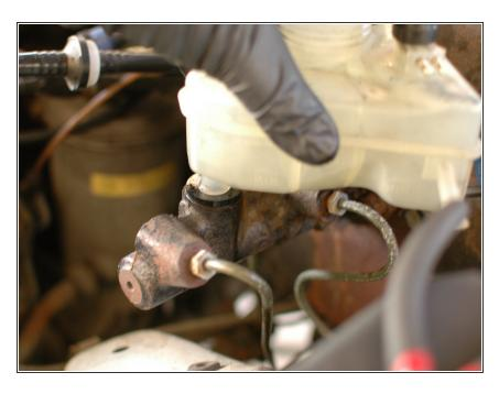
Now you can push the brake reservoir in to the front plug opening. Do this with the reservoir at an angle from the master cylinder.
