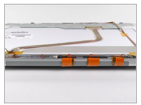
Remove the five Phillips screws securing the clutch cover to the bottom edge of the front display bezel.
