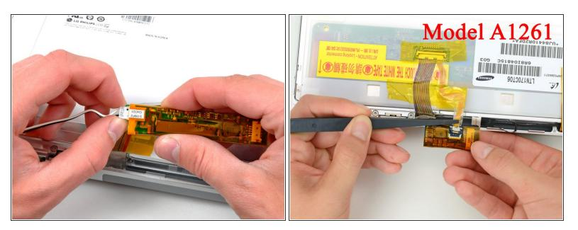
• Disconnect the backlight connector from the inverter board.
