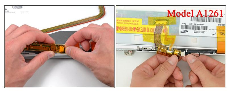
• Disconnect the inverter cable by pulling its connector away from the socket on the inverter board.
