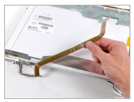
• Remove the display data cable from the display assembly.
