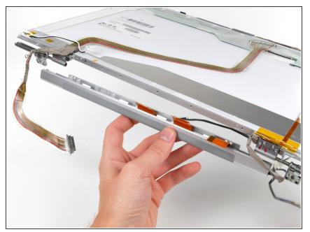
• Remove the clutch assembly from the front display bezel, minding any cables that may get caught.
