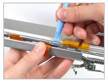
Repeat the process covered in the previous step to free the other side of the clutch assembly from the front display bezel.
