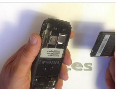
Switch off the device and remove the battery for 5 sec.
