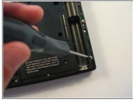
Using a Philips Screwdriver #00 unscrew the twelve 11.8mm screws shown in the picture and located on the back of the calculator.
