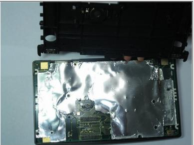
Now pull up on the back cover of the calculator while holding the rest of it flat on a surface.
