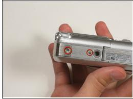
Remove five screws from the camera casing using a tri-point Y0 screwdriver.
