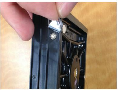
Note the label: Warranty Void If Seal Broken. In this case, we want to retrieve the data and do not care about the warranty. Remove the label, to expose one of the four total screws on the side to remove the internal drive.
