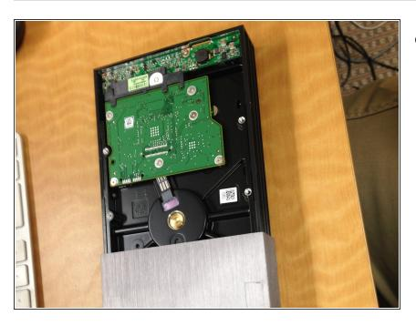
Carefully push on the front, black faceplate to slide the drive and housing out of the case.
