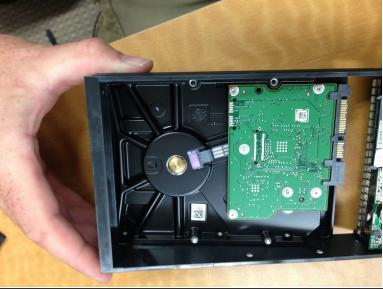
Carefully remove the four screws holding the drive in the caddy, making sure that the hard drive does not slip out or damage the SATA controller card towards the rear of the case.
