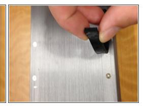
Turn the drive over, noting the black rubber strips. Carefully peel each strip off, to reveal a set of two phillips screws under each strip.
