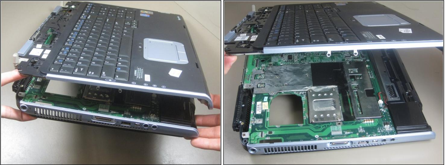
**⚠ Do not remove the keyboard yet! There are still wires connecting the two components.**
