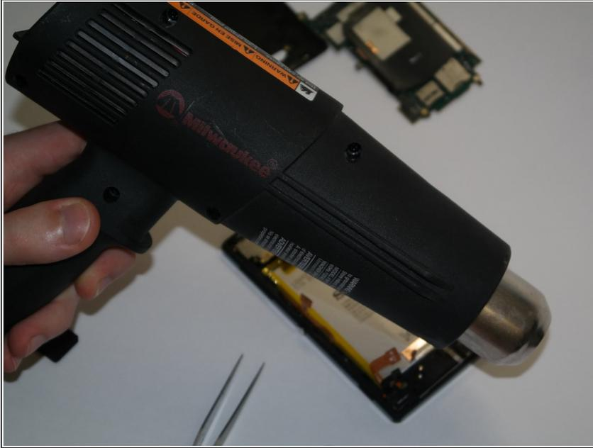
**⚠** The objective is to remove the battery with the least amount of stress possible. Although it may not be likely on its own, **bending lithium-polymer batteries will break their internal seals, and CAN EVEN CAUSE THEM TO EXPLODE!**
