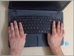
• The Keyboard is held by 7x locking clips. Use cutter and plastic tools to unlock them.
