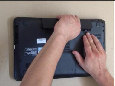
Switch-off the laptop and remove the battery.
