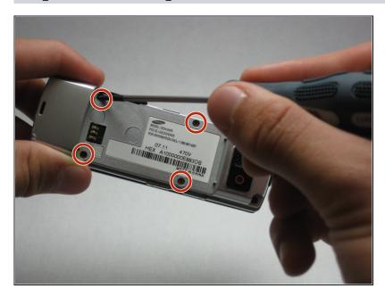
Remove the four screws from the back of the phone using a Phillips #00 screwdriver.
