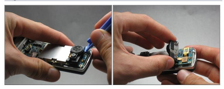
• Use the iFixit opening tool to remove the camera/speaker from the motherboard.
