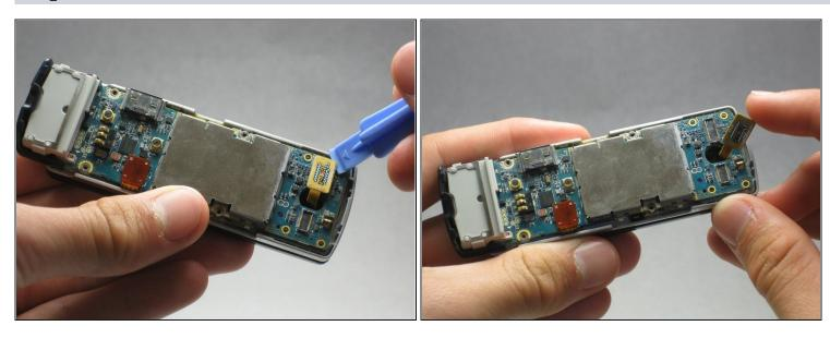
• Use the iFixit opening tool to remove the yellow tab on the motherboard.
