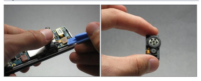
• Use the iFixit opening tool to gently pry the camera/speaker off.
