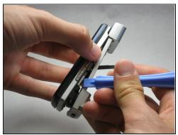
• Locate the USB port (where the charger can be plugged in). Using the iFixit opening tool, open the phone cover.
