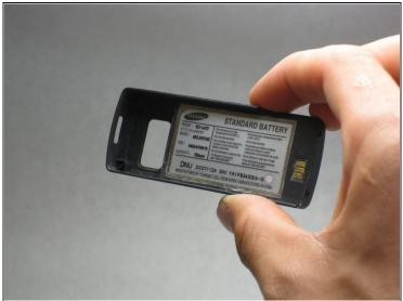
• While holding the button down, remove the back cover of the phone.
