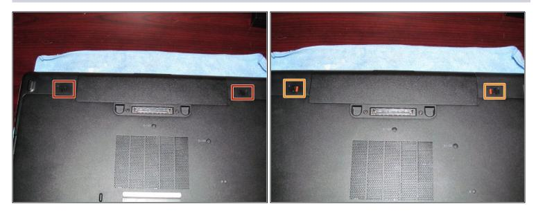
Flip the laptop over and unlock the 2 battery tabs. The tabs will remain unlocked until the battery is removed.
