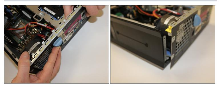
• While rotating the case-opening knob, slide the motherboard tray away from the front of the computer.
