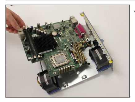
• The motherboard can now be removed from the remaining panel.
