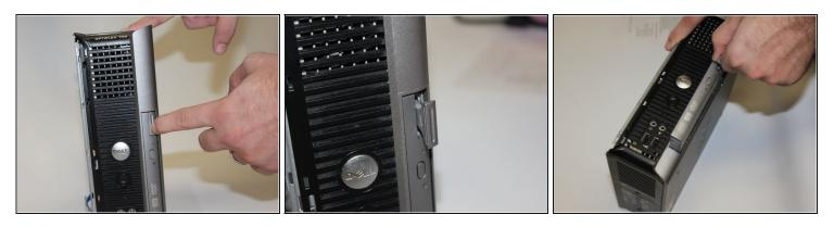
• Press the large button on the corner of the optical drive. Pull on the pop-out button to slide the optical drive out.
