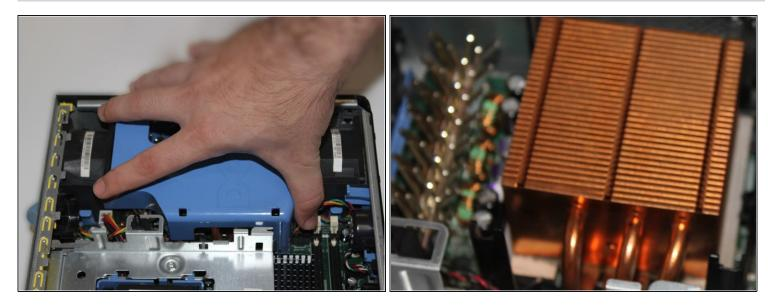
• Remove the blue shield by sliding it straight upwards.
