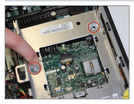
Remove two silver 6mm #2 Philips screws from the Hard Drive Stand.
