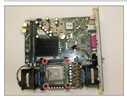
Remove the four black 9mm #2 Philips screws located on heat sink stand.
