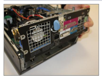
• Lift the motherboard from the rest of the computer case.
