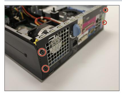
• Remove four black 6mm #2 Phillips screws located at the back of the computer tower.
