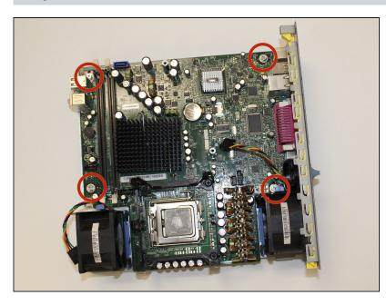
• Remove the four silver 6mm #2 Philips screws holding the motherboard to the rear computer panel.
