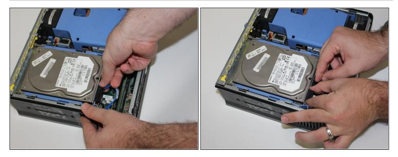
A Ground yourself to avoid static from damaging any components. Either use a wrist strap and antistatic mat, or touch the metal computer case every few minutes.
