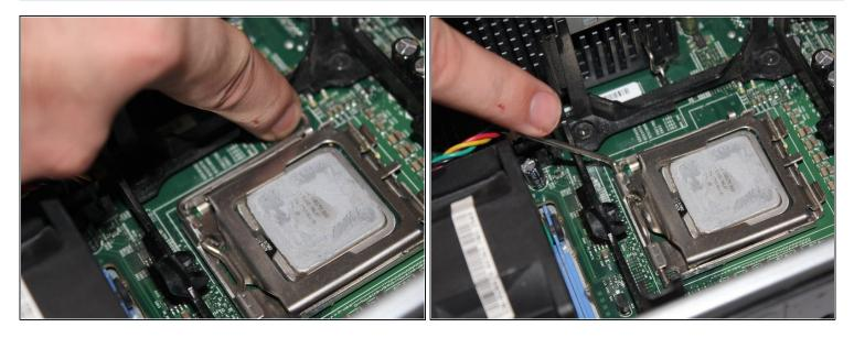
Ground yourself before removing any internal components.
