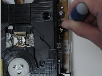
Remove the four screws around the DVD drive with a phillips head screwdriver.
